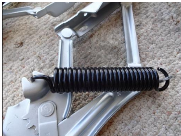
Above: Freshly reconditioned hinge assembly ready for installation on a ‘57 Safari wagon. They were cleaned and painted without chemicals or sandblasting, then painted. They work great!
