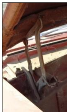
Above: ‘55 hinge assembly looking tired and making noise but it’s still holding-up the hood.
