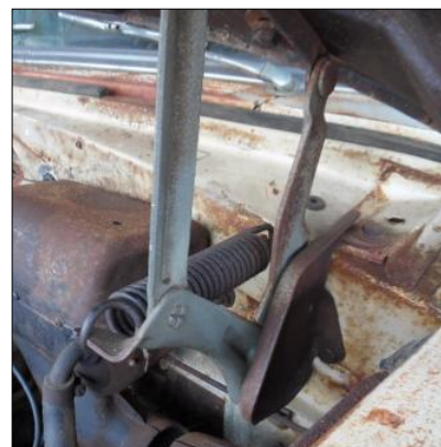
Above. ‘56 hinge assembly shown before the owner applied oil. It was weak and noisy. Afterwards, the hood would not stay open but it was quiet!
