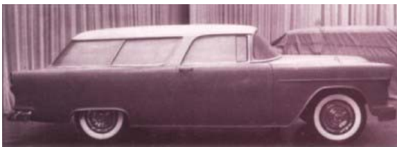
By March 11, 1954, design work was largely completed, though the rear wheel openings seen here are much smaller than on the production Nomad.
