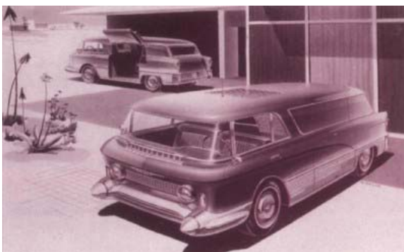
A design study, the GMC Expedier van embraced the Nomad/Safari hardtop styling and slanted B-pillars.
