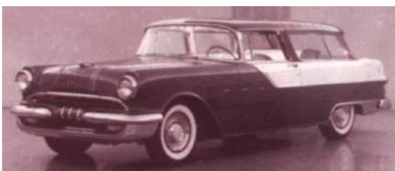
The 1955 Pontiac Safari shared its greenhouse, front doors, and tailgate with the Chevrolet Nomad.
