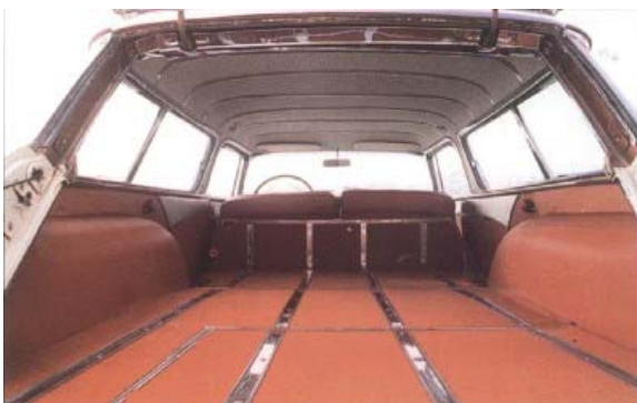
Pontiac Star Chief Safari cargo capacity with the rear seat up was 36 cubic feet, but when down this expanded to a more useful 71 cubic feet.
